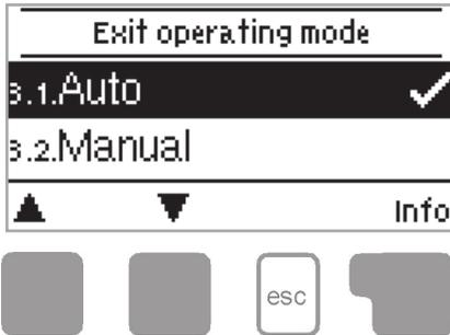
In the menu "4. Operating mode" the controller can either be placed in automatic mode, switched off or placed in a manual operating mode.
