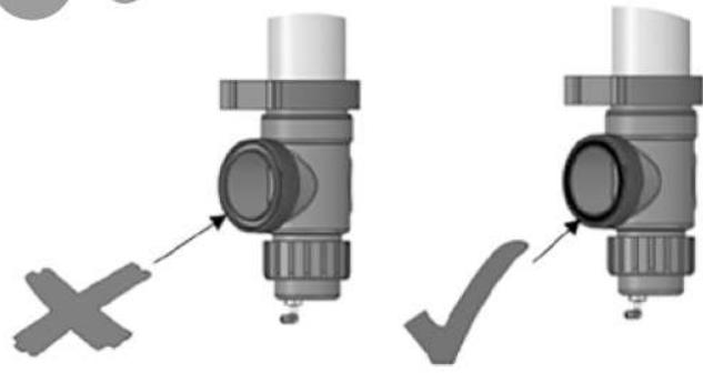
Make sure the O-ring is in the correct position.
